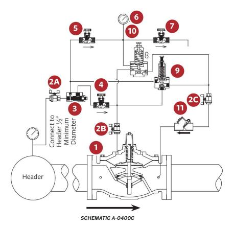
**Note:** Schematic shown is for 50 mm to 150 mm. For 200 mm and higher refer to Schematic A-0401C
